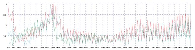
\*Red VSWR measured with no ground plane with with 2m (6'6") of RG174 cable.
