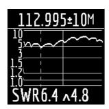
at the top of the screen: the value of the center frequency of the measurement and the width of the measurement band. in the middle of the screen: SWR chart
