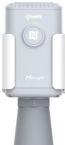
EM500-UDL is designed for objects distance or level detection in harsh environments and transmitting data using LoRaWAN® technology. With this low power consumption technology, EM500-UDL can work up to 10 years with 19000 mAh battery. Combining with Milesight LoRaWAN® gateway and Milesight IoT Cloud solution, users can manage all sensor data remotely and visually.
